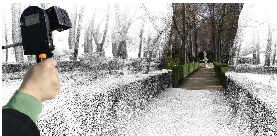
Figure 2. The MLS sensor contributed effectively to acquiring the 3D point cloud. A new topographic map has been generated to meet the need to update the tree inventory in a historic garden. This is an agile and powerful tool for the management and maintenance of a protected space.
