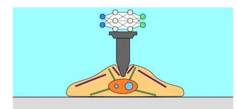
This tool is designed for fast processing of atomic force microscopy (AFM) data and to extract nanomechanical properties of soft samples such as polymers, cells or tissues in their native state.
