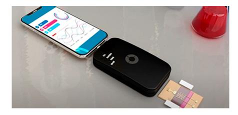
Portable diagnostic device for the detection of analytes in biological samples. The biosensor allows a label-free quantitative detection. Simple use, no qualified personnel needed.
