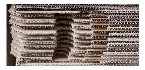
Reinforced packaging paper exhibiting a surprising increase in compression strength and stiffness, obtained through the application of a bio-product obtained from ligno-cellulosic waste, without the need to add cellulosic fibers, strength additives or subjecting the paper to additional manipulation.
