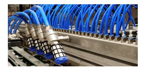
Resistant and flexible valve for pneumatic flow control in fluid circuits. Its monolithic structure prevents failures caused by defective parts, and is also cheap to produce and easy to install and replace. It can be used without the need for a direct electrical connection.
