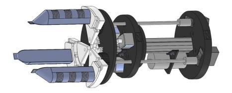
Grip with soft actuators specifically designed for handling delicate objects without damaging them, with independent actuators that allow for an adapted (and real-time adaptable) gripping, being therefore of special interest in automated harvesting tasks.
