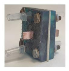
New compact electrochemical device that can be adapted to different applications such as: flow cell, fuel cell or electrolyzer to produce H<sub>2</sub>.
